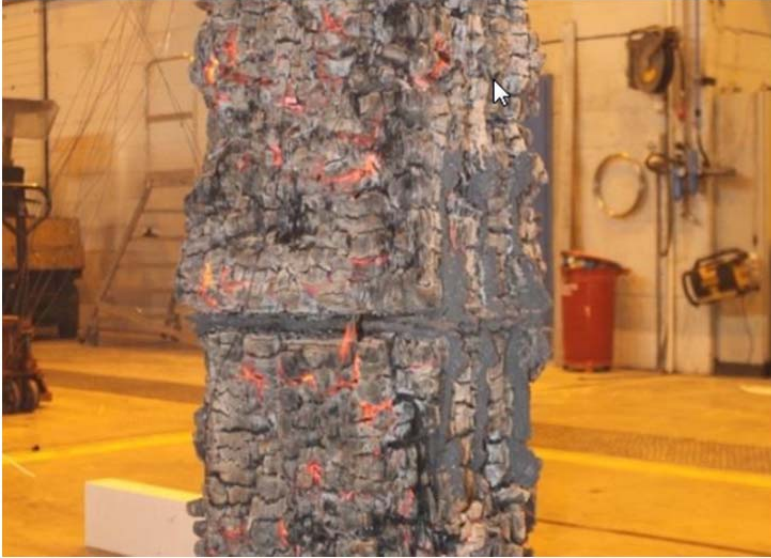
Figure 5 Fire test of glulam at SP Firetech. Standard ISO fire for 90 minutes and observation in the cooling process. This specimen has an internal steel connection
