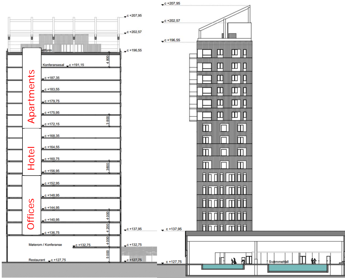
Figure 12 Typical sections for Mjøstårnet. Please note that the final elevations are somewhat different to what is shown here
